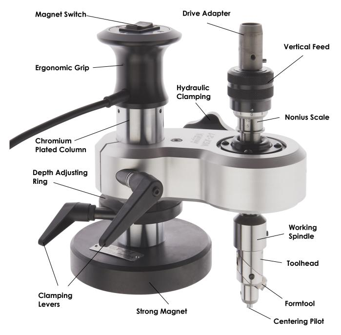
The portable VGX-21 valve seat refacing unit has been developed for the specialised petrol and diesel cylinderhead workshop. The highly accurate valve seat processing is achieved by a spherical spindle guide bearing as well as a unique **hydraulic ball clamping system**. A almost pressure free centering and braceless fixing of the MIRA® rotary head is made possible in order to achieve precise and concentric valve seats!
