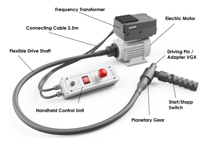
The new **VARIO-DRIVE EVO** significantly improves the efficiency of your cylinderhead workplace. The unit enables a fatigue-free and time saving refacing of valve seats and counterbores and guarantees a smooth and even cutting motion. The new **VARIO-DRIVE EVO** is well adapted to complete all hand-driven MIRA Valve Seat Units.
